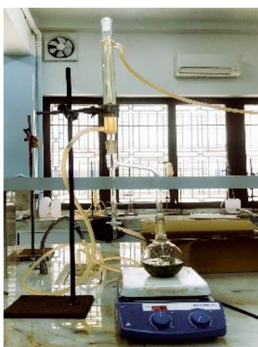
Fig. 2. Hydro-distillation system used in this study
