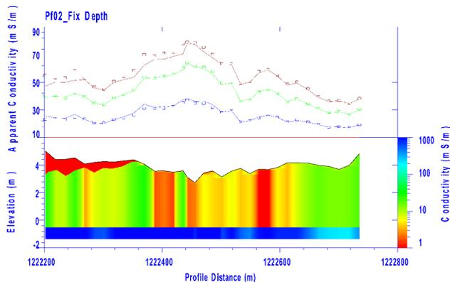
**Fig. 7.** Apparent ground EC inversion with a 3 layers model for 1 profile (P02-Fixing depth) between prek Chann and prek Touch in IX1D software
