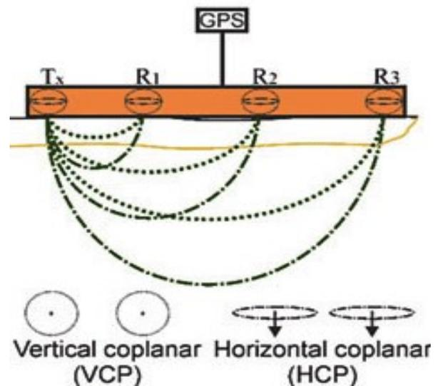
**Fig. 2.** Collecting ground EC with electromagnetic sounding
