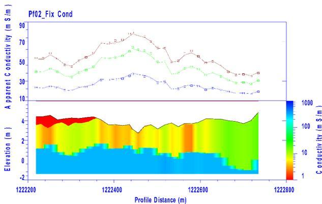
**Fig. 6.** Apparent ground EC inversion with a 3 layers model for 1 profile (P02-Fixing cond) between prek Chann and prek Touch in IX1D software
