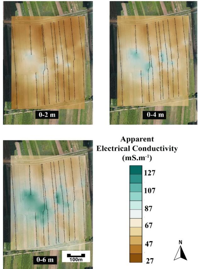
Fig. 5. 2D mapping of the ground EC between prek Chann and prek Touch (June, 2022)
