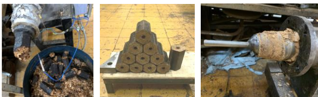
Fig.2. (a) Unshape production, (b) Certified briquettes, (c) Operation failed
