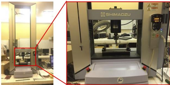
Fig. 5. Three-point bending test operated on specimen by AG-Xplus series Autograph universal testing machine
