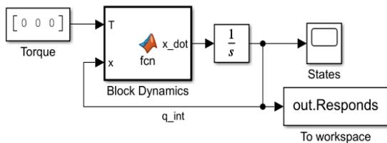
Fig. 5. Open loop Simulink model
