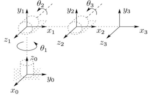
Fig. 2. The general coordinate set by the DH method (Kucuk & Bingul, 2006)
