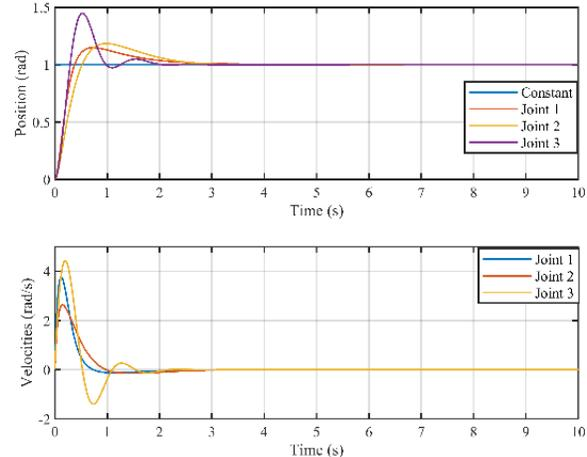
Fig. 8. The response of the closed-loop system with a constant 1 and its derivative is used as an input
