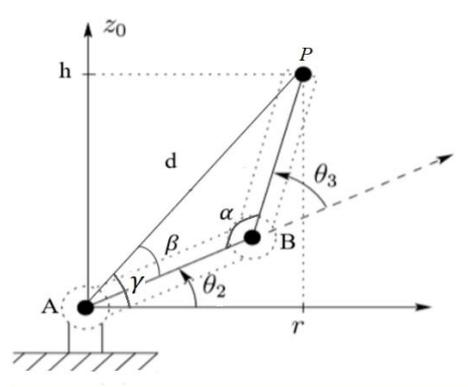
Fig. 4. Plane geometry for determining the variable of joints 2 and 3
