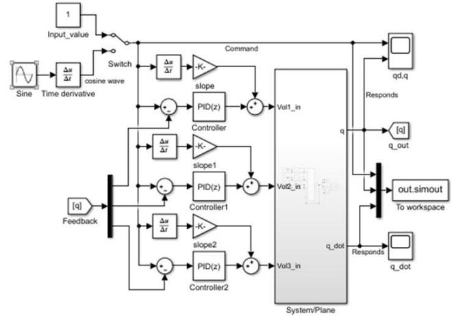
Fig. 7. Closed-loop Simulink model with PID controller
