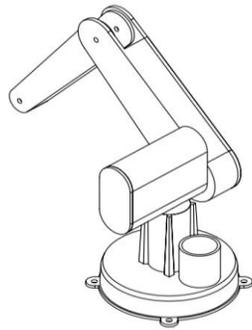
Fig. 1. 3-RRR robot manipulator in 3D view
