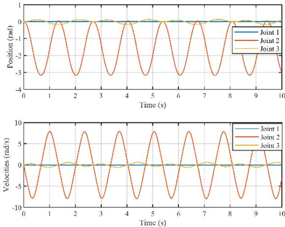
Fig. 6. The opened loop response with zero torque was applied
