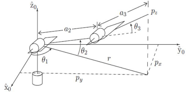
Fig. 3. Inverse position of the robot (Lynch & Park, 2017)
