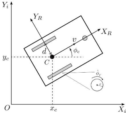
Fig.1. A Differential Drive Mobile Robot
