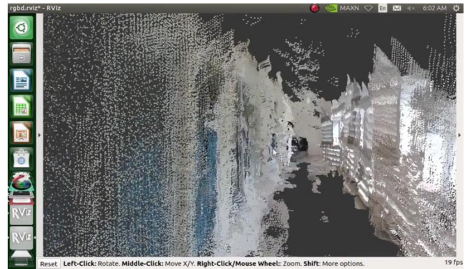
Fig. 11. Indoor 3D mapping in the detailed point cloud
