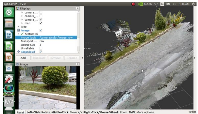
Fig. 12. Result of 3D mapping (Outdoor)
